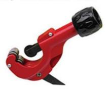
Used for removing the outer sheath(PVC & Plenum types) of fiber optic cable
